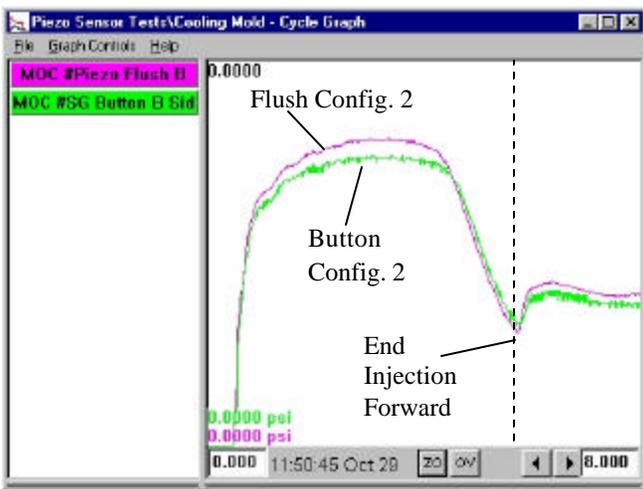
Figure 7: Example of Cavity Pressure Profiles Using Configuration 2
