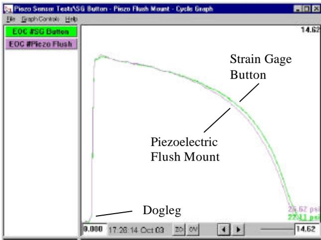
Figure 3: Example of Cavity Pressure Profiles: Configuration 1
