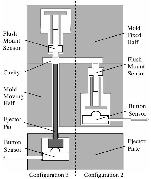
Figure 2: Illustration of Configuration 2 (Button Beneath Direct Sensor) and Configuration 3 (Direct Sensor Across from Moving Ejector Pin)
