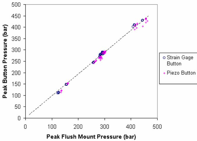
Figure 5: Correlation of Peak Cavity Pressure Data Using Configuration 1
