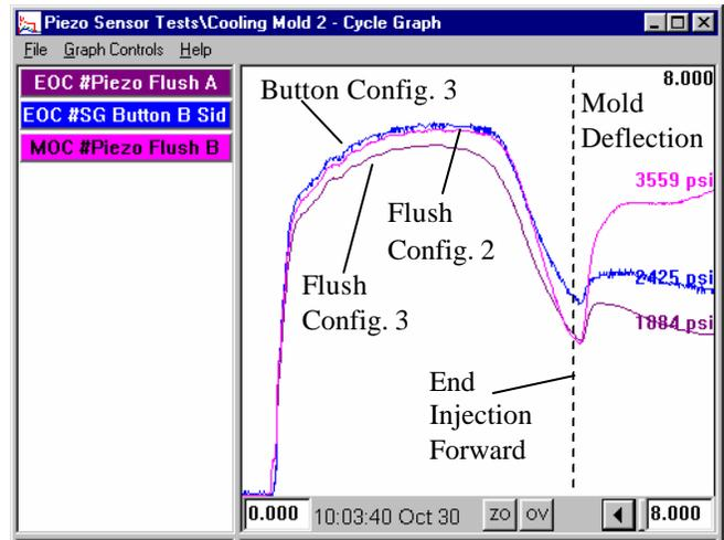
Figure 8: Example of Cavity Pressure Profiles Using Configuration 3
