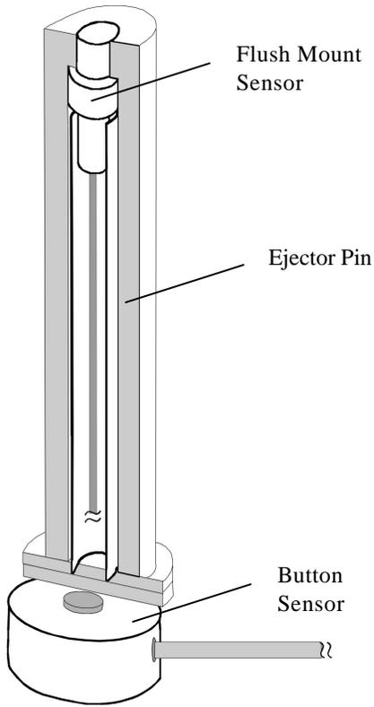
Figure 1: Illustration of Configuration 1: Direct Sensor Installed in Moving Ejector Pin
