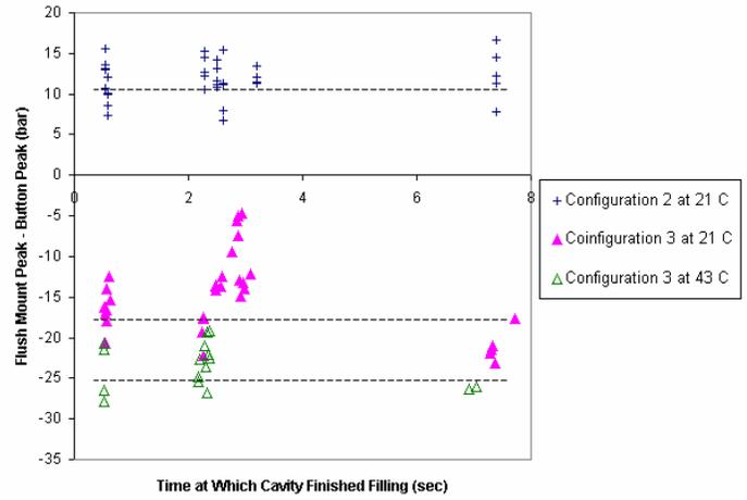
Figure 6: Difference in Peak Data Between Sensors Using Configuration 2 and Configuration 3
