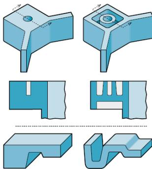
Also, remember that sharp corners cause stress concentrations in molded parts. If you must make transitions in wall thickness, gradual transitions can help reduce pressure losses through the part, giving better overall dimensional control.
